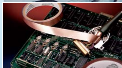
EMI-RFI copper tape shielding
