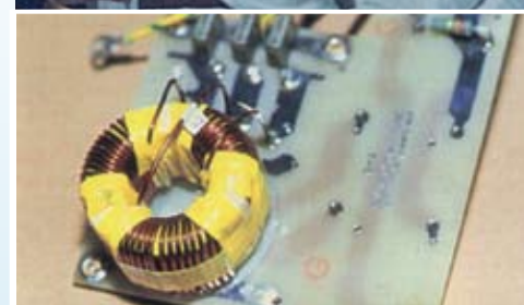
Coil outer wrap taping
