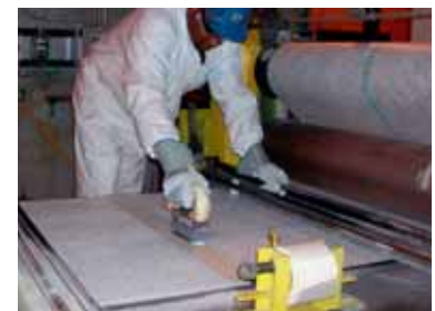
Machine operator using CHR G-476 in roofing production plant for substrate/carcass splicing.
